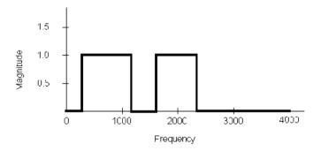
The desired weighting specifications for the magnitude response of this filter conform to the following specifications using the polynomial magnitude format:
