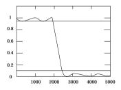
An Elliptic filter is based on a mapping of the following function:
